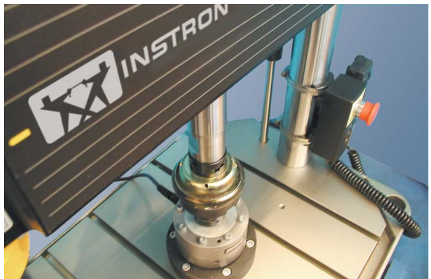
▲ An engine mount is tested on an Instron 8872 machine
